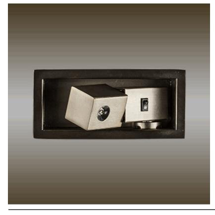
6-3/4" Antique Bronze Wall Lamp, 3 watt integrated LED, 12' black cord with in-line driver, on/off rocker switch, designed to mount in a headboard on the left side of the bed
